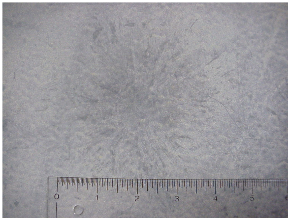
Photo 6, 3" Ice Sphere, 20 ga. Metal, 90 degree impact
