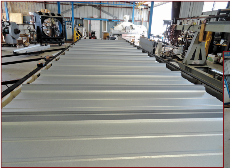
Figure 4 – Roof panels mounted on purlins prior to base testing.
